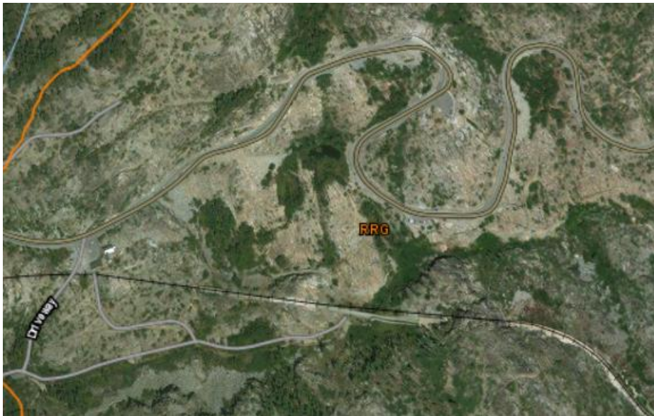
Figure 3.1 Soil Map of Summit Camp area. RRG= Rock outcrop, granitic-tinker complex, 30 to 75 percent slopes. Map generated with USDA web soil survey.
